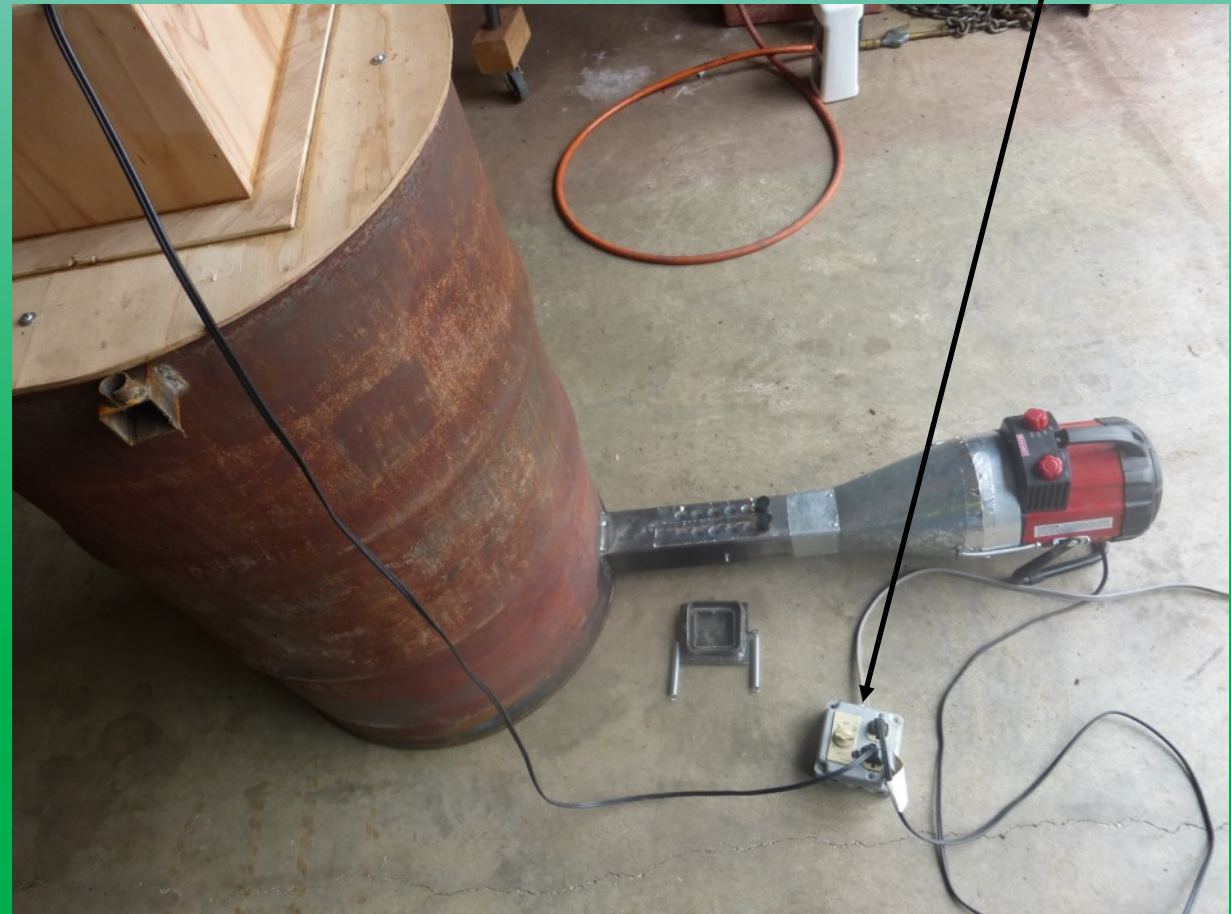
Spring wound Timer to turn off the fan and dryer
