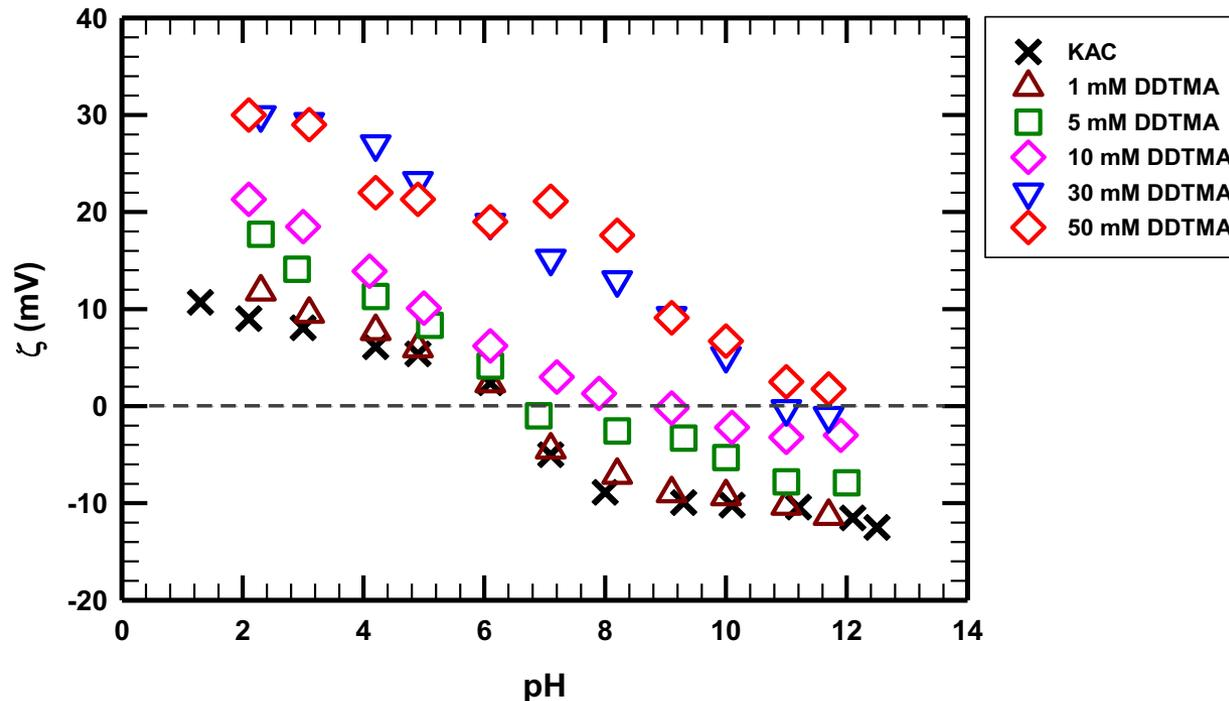
**Zeta potential of functionalized KAC functionalized with HTMA, OTMA, DCTMA, DDTMA, TDTMA, and HDTMA.**
