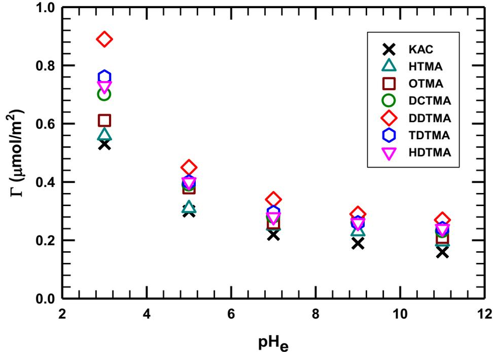
**Effect of pH on fluoride removal by functionalized KAC functionalized with HTMA, OTMA, DCTMA, DDTMA, TDTMA, and HDTMA.**
