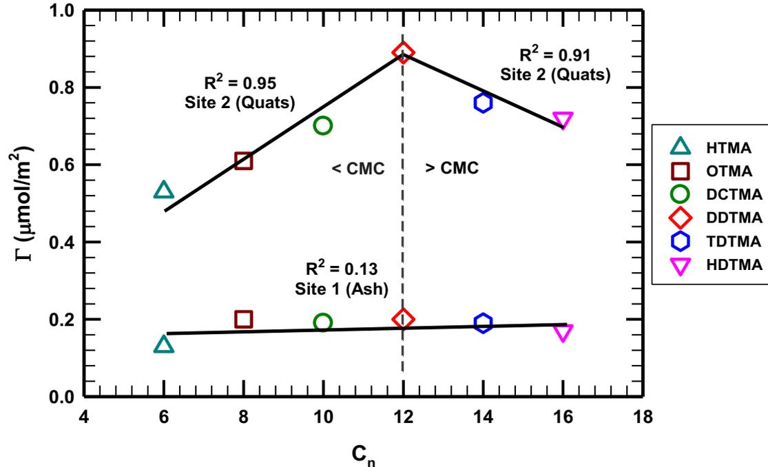
**Adsorption of fluoride on KAC functionalized with HTMA, OTMA, DCTMA, DDTMA, TDTMA, and HDTMA.**
