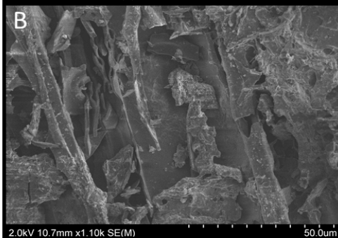
B) Biochar after 1 year in the bag from the Oxisol napiergrass plots
