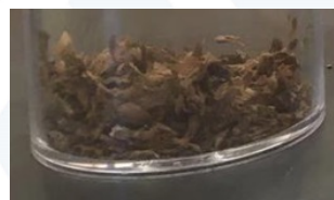
Lignin extraction for 2 hr at 140 °C
