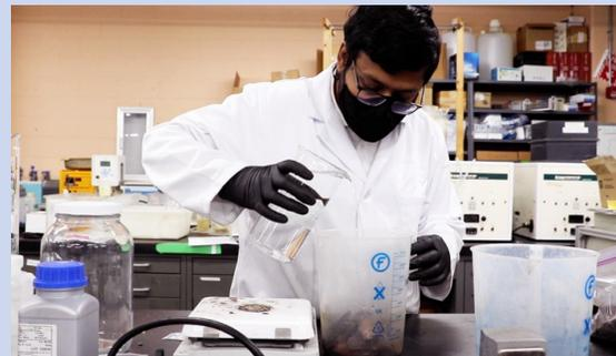
*Nitesh Kasera is studying the effect of nitrogen doping on >> biochar and its ability to remove nitrate and phosphorus from aquacultural wastewater.*
